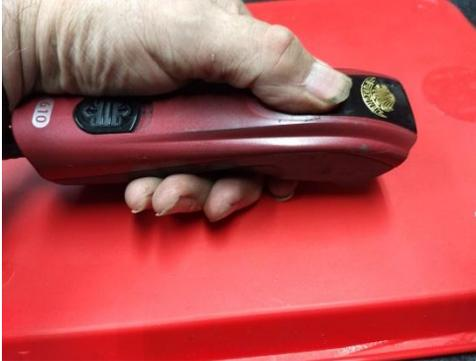
Removing the logo plate is step one. If you already have the Furzone 610, and have changed the lever, your already ahead of the game. The logo board slips off just like the battery cover on your TV remote. Push forward, then lift up from the front. It has little tabs that lock it in on both sides. Watch how this cover comes off, because the vac attachment goes back on the same way. See where the rear tabs go as well.
