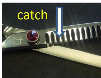
These blades are actually two razors going back and forth, and they need to be close. The tension wheel is not there to adjust the tension for scissoring convenience, its there to adjust the shears so they cut properly. Loosening the tension too much can cause a catch 1" from the pivot, or hair to fold near the front. Always lube the pivot with shear lube only NO BLADE OIL. You can get shear lube at any beauty supply store.
